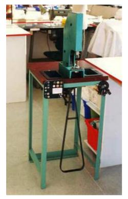
KPR1 is a foot operated ratchet press. It is supplied complete on a stand which incorporates two side trays for stud part storage. It is designed to attach most press fasteners, rivets eyelets, jeans buttons etc.
